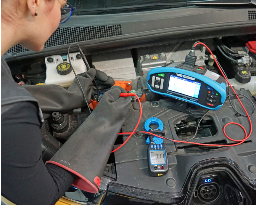
Measuring the simulated insulation problem with MD 9070 and reference resistance A 1734.
