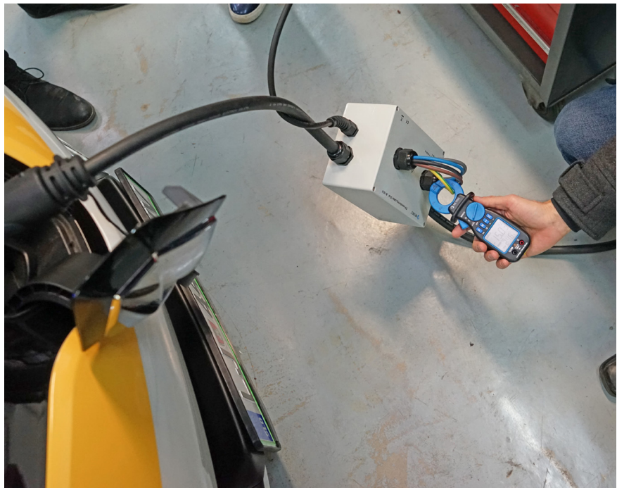
Testing the leakage current in PE wire while charging the car.
